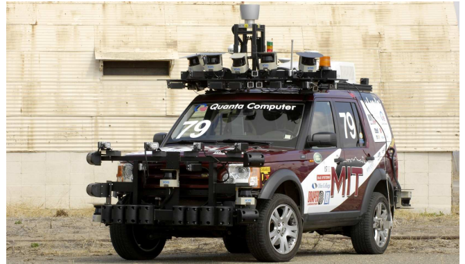
Fig. 1. The MIT Urban Challenge vehicle used to capture the presented data set. The vehicle is equipped with a high-precision GPS/INS, calibrated cameras, SICK laser range scanners, and a Velodyne 3D scanner.
