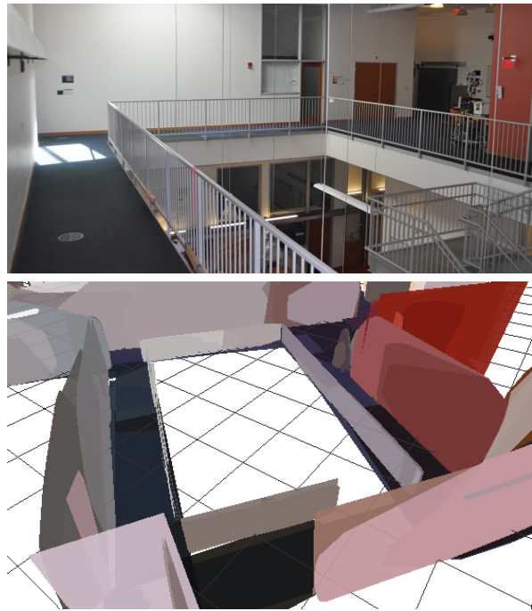
Fig. 2. The first step of this algorithm is to generate a 3-D building model which indicates the broad geometric information (but not the precise textural information). Plane colors are for illustration purposes only at this stage. This model is later used to allow an RGB-D sensor to localize.
