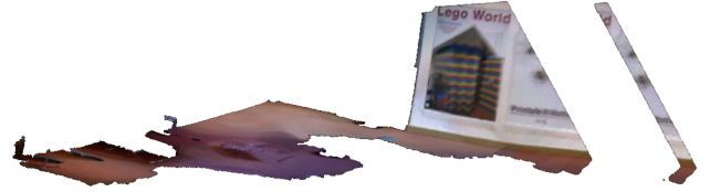
Fig. 3. Example iteration step for adding new data to a map. On right: the new data to be added to the existing map. Left: the new data and the segments that were suggested to be redone after the first iteration. The first segments joined are the wall and floor segments that the new data was adding to.
